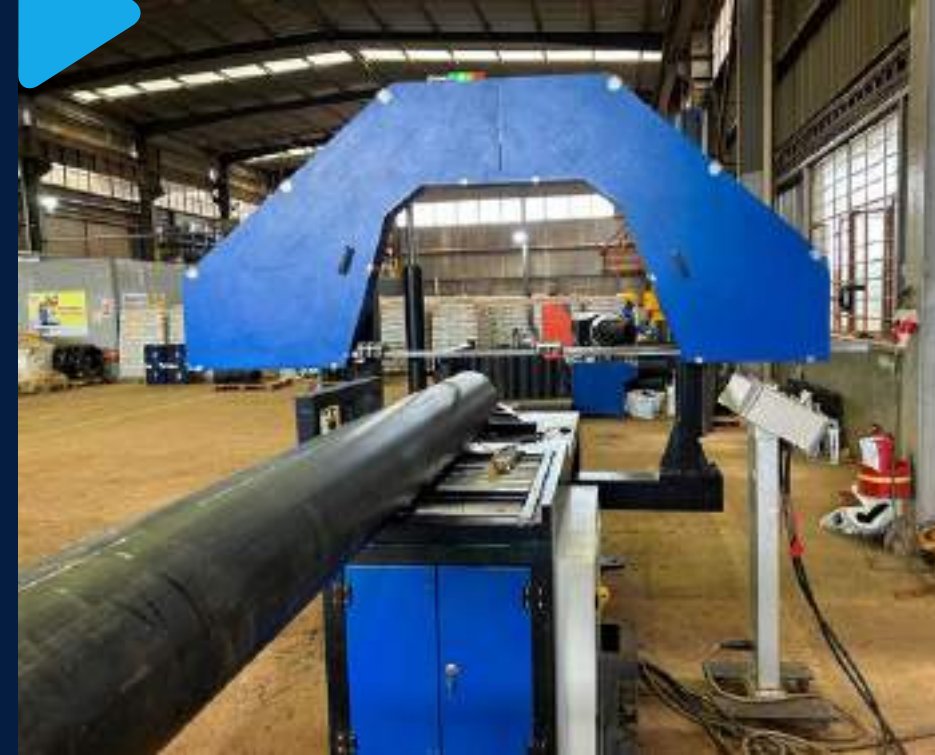
Multi Angle Pipe Cutter
