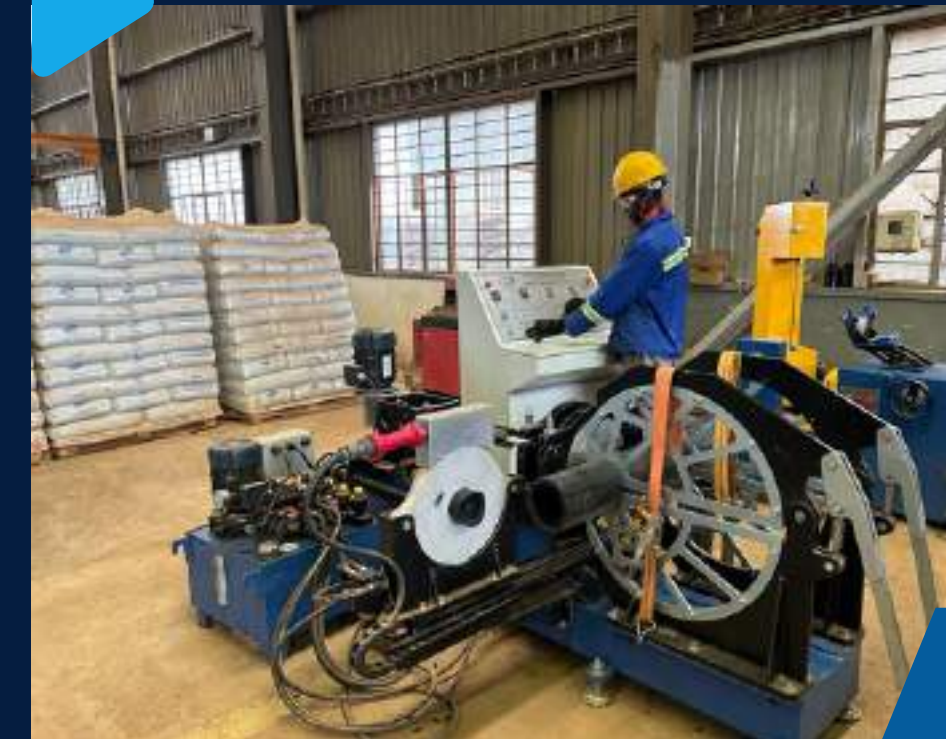
Saddle Fusion Welding Machine
