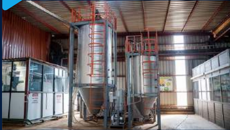
Line 1 : High Efficiency Resin Drying Tower
