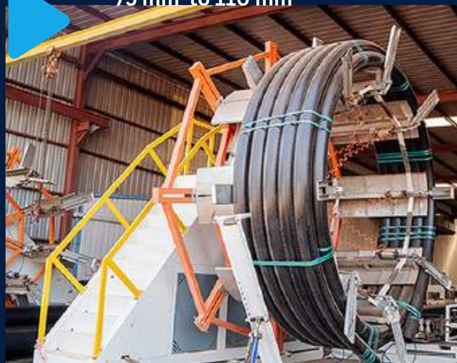
Single Station Pipe Winder -3 110 mm to 180 mm
