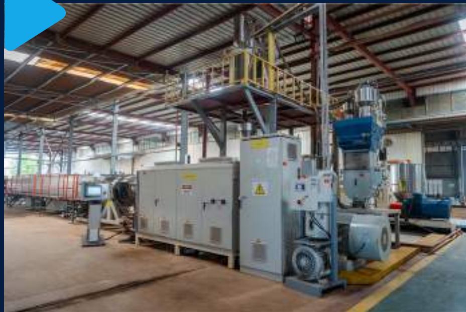
Line 2 : Extruder 315 mm up to 630 mm
