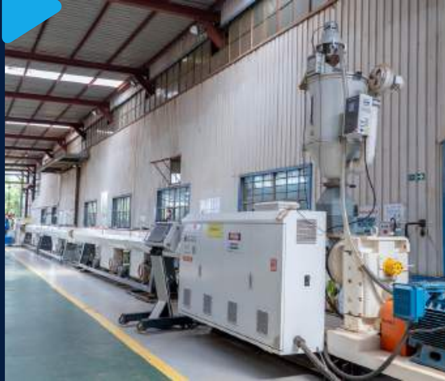
Line 4 : Extruder & Downstream 20mm to 110 mm OD
