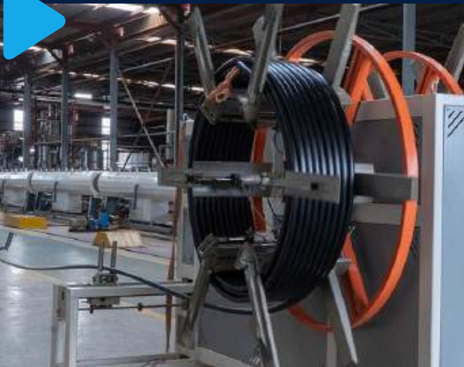
Line 4 : Extruder & Downstream 20mm to 110 mm OD
